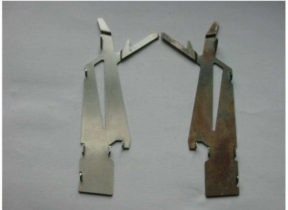
Further, To remove all traces of such heat treatment and any other addition of chemical elements (especially in corners and edges etc. and restore the section to the original finish is nigh on impossible.
